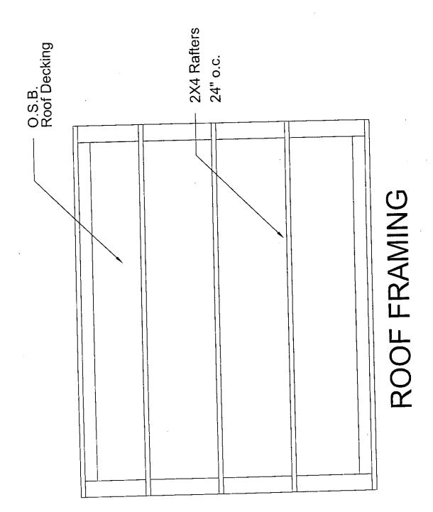
The equivalent ground snow load per ANCE 7-97 is 68 PSF which exceeds the 16.2 PSF pressure for a NOTES: 1) The Roof System of this, 10 ft. wide Gabrel style building has a live load capacity of 35 PSF.
